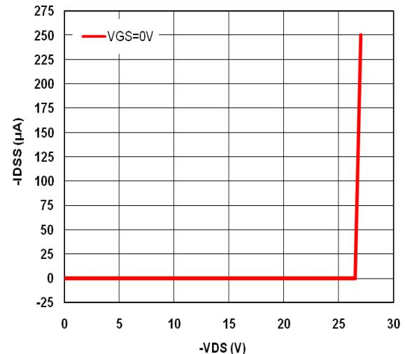
**Fig6. IDS vs. Drain-to-Source Voltage**
