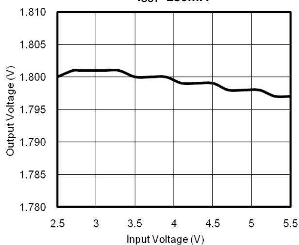
Output Voltage vs. Input Voltage I_{OUT}=150mA
