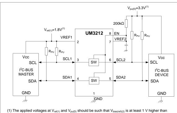
(1) The applied voltages at V<sub>ref(1)</sub> and V<sub>pu(D)</sub> should be such that V<sub>bias(ref)(2)</sub> is at least 1 V higher than V<sub>ref(1)</sub> for best translator operation.
