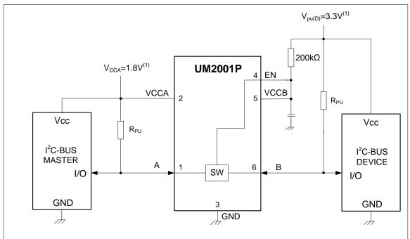
(1) The applied voltages at  $V_{\text{CCA}}$  and  $V_{\text{pu(D)}}$  should be such that  $V_{\text{CCB}}$  is at least 1 V higher than  $V_{\text{CCA}}$  for best translator operation.
