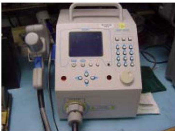
Figure 5. ESD Generator, NoiseKen ESS-2000
