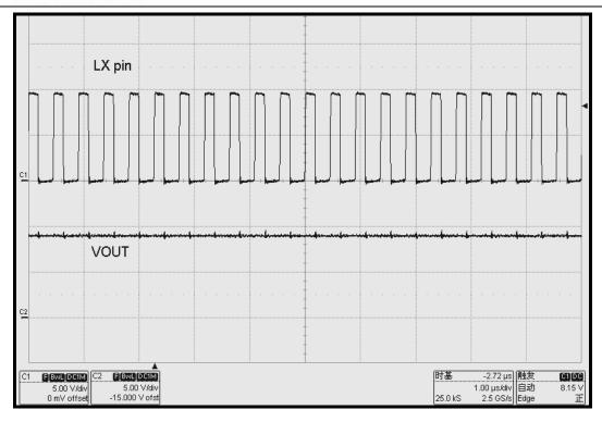
Fig 2.1 Output waveform diagram (Vin=3.6V, 3 pcs LED load)
