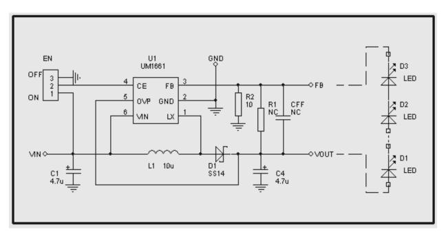
Fig 1.1 UM1661 EVB board schematic
