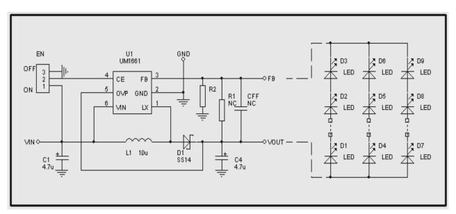
Fig 5.1 UM1661 EVB board driver multi-string LED
