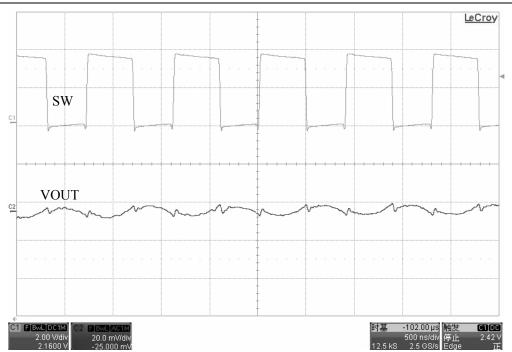
Fig 2.1 UM3501 waveform diagram (V<sub>IN</sub>=3.6V, V<sub>OUT</sub>=1.8V, I<sub>LOAD</sub>=300mA)
