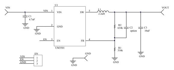
Fig 1.1 UM3501 EVB schematic (Recommended Value of R1 and R2 for 1.8V output)
