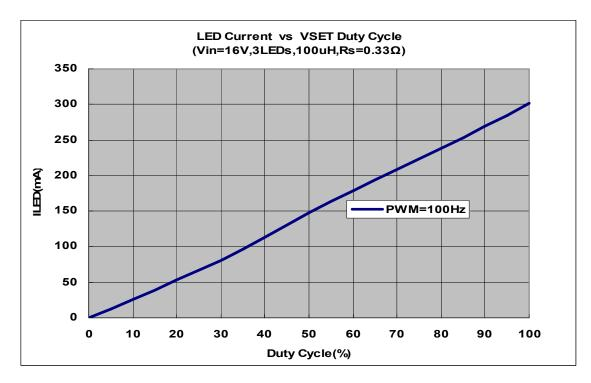
Fig 2.3 PWM Dimming
