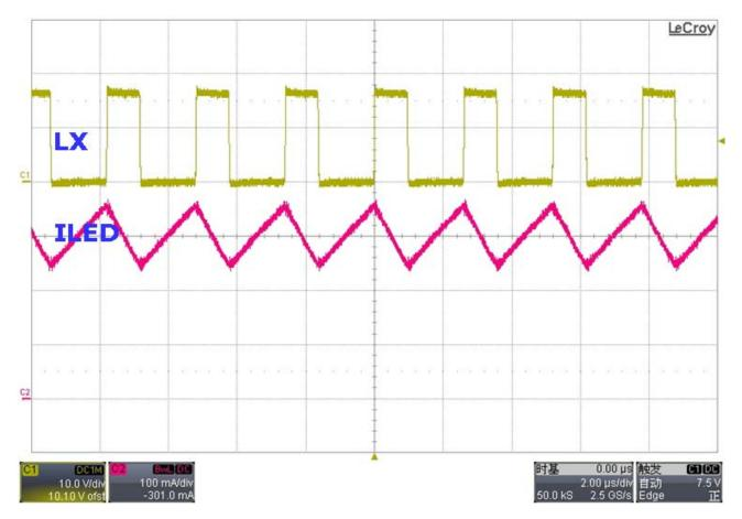
Fig 2.1 Typical Switching Operation Waveforms (3 LEDs,100uH,Vin=16V,Rs=0.33  $\Omega$ )
