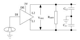
Figure 3. Driver Timing Test Circuit
