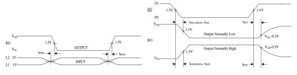
Figure 9. Receiver Propagation Delays
