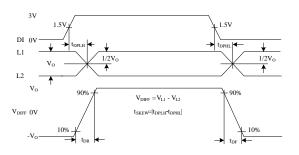
Figure 7. Driver Propagation Delays
