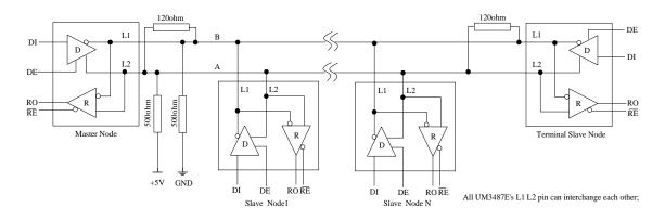
Figure 1. Typical Half-Duplex Non-Polarity RS-485 Network
