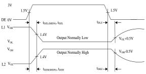
Figure 8. Driver Enable and Disable Times
