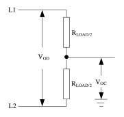
Figure 2. Driver DC Test Load
