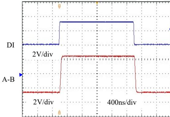
**Receiver Propagation Delay**
