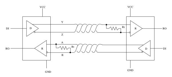
Figure 1: UM13087S8 pin configuration and typical full-duplex operating circuit
