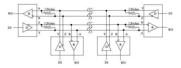
Figure 2: Typical Full-Duplex RS-422 Network
