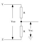
Figure 3. Driver DC Test Load
