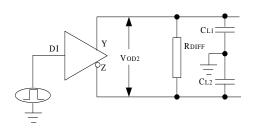
Figure 4. Driver Timing Test Circuit
